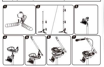
Stand components include three poles of different lengths to adjust height. You can choose a suitable height from seven combinations.
